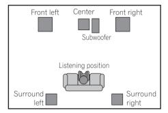
• Front surround 3-spot setup – This setup is ideal when rear surround speaker placement isn't possible or you want to avoid running long speaker cables in your listening area. Use this setup together with the Front Surround modes to take advantage of wall and ceiling reflections for a very realistic surround effect.
